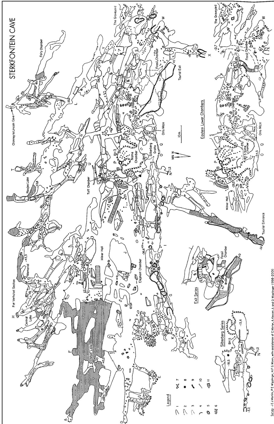
**Fig. 2.** Map of Sterkfontein Cave. **Legend:** 1) cavity outline; 2) cavity outline under single overlay; 3) cavity outline under double overlay; 4) scarp and edge of pit in cave; 5) scarp and edge of pit at surface (=entrance); 6) blocks and scree; 7) walls of breccia and boulder blockages; 8) *Australopithecus* skeleton; 9) masonry wall; 10) gates and fences; 11) flight of stairs.
